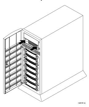
Figure 5 Remove Screws to Release Controller from Housing
