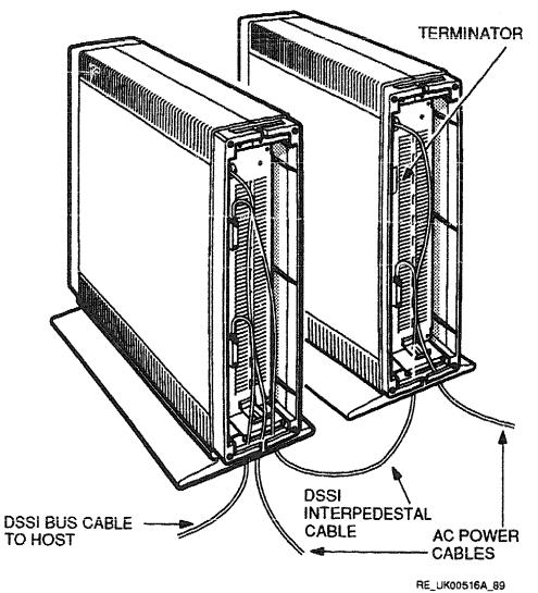
Figure B-3 Interpedestal Cabling
