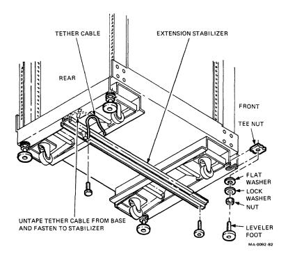
Figure 6-5 Cabinet Leveler Feet Assembly and Extension Stabilizer
