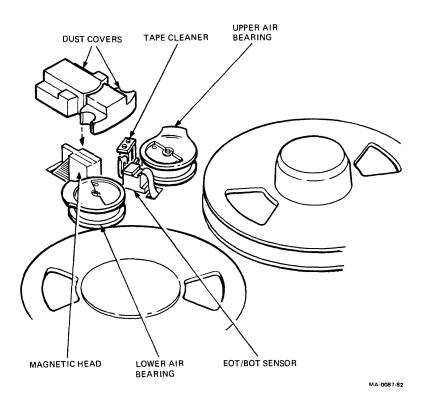
Figure 4-2 Magnetic Head/Tape Path Components
