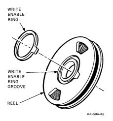
Figure 2-2 Write-Enable Ring
