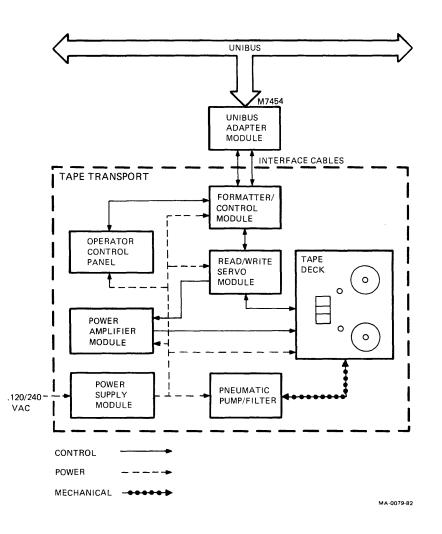
Figure 1-3 TU80 Functional Diagram
