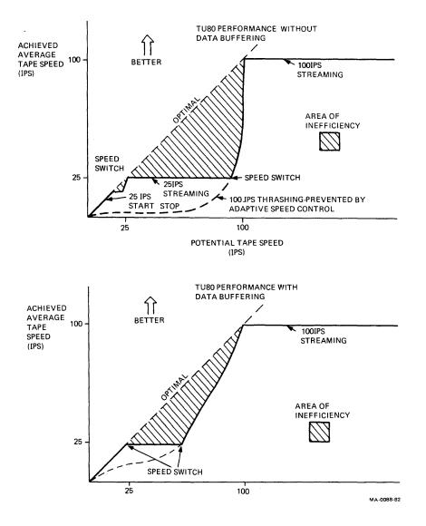
Figure 5-1 Data Buffering and TU80 Performance Upgrading
