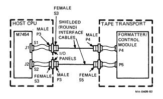
Figure 6-11 Plug-to-Plug Connections of I/O Cables
