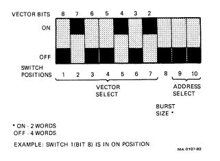
Figure 6-14 DIP Switchpack Setting for a Single TU80 Configuration (Address 172522, Vector 224)
