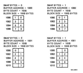
Figure 5-7 Byte Swap Sequence, Forward Tape Direction (Read or Write)
