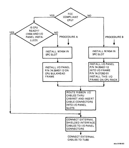
Figure 6-15 TU80 Interface Cabling Flowchart
