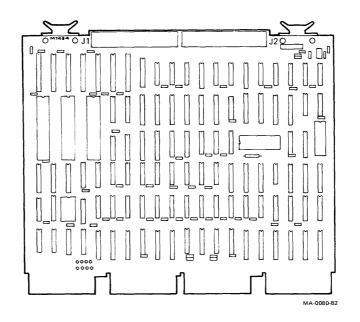
Figure 1-4 UNIBUS Adapter Module M7454
