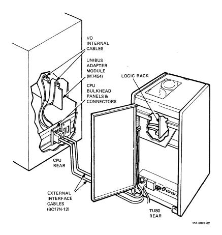
Figure 6-10 Typical Interface Cabling
