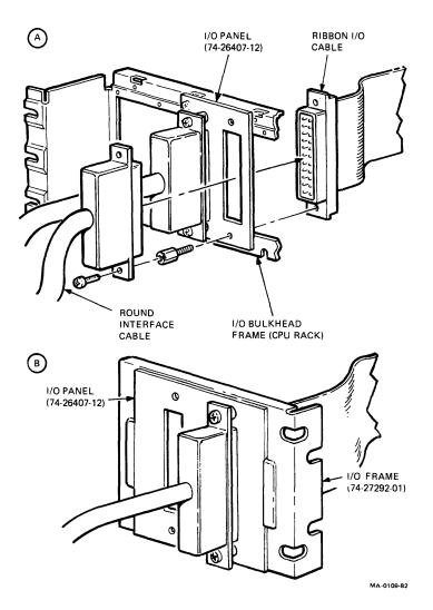
Figure 6-16 I/O Bulkhead Connector Panel and Frame
