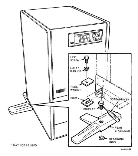
Figure 6-8 Rear Stabilizer Installation
