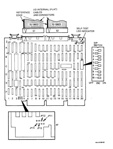
Figure 6-13 UNIBUS Adapter Module and I/O Internal Cables
