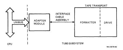
Figure 1-2 TU80 Subsystem Block Diagram
