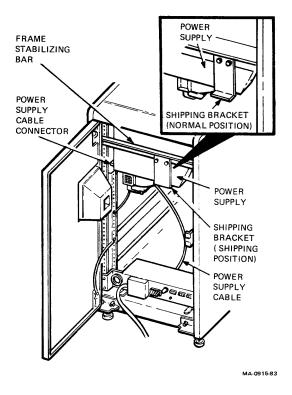
Figure 6-4 Reversing the Rear Shipping Bracket
