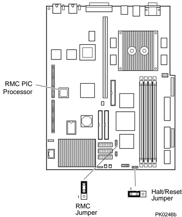
The RMC logic is implemented using an 8-bit microprocessor, PIC17C44, as the primary control device. The RMC PIC is programmed with code to control access to various environmental status bits.
