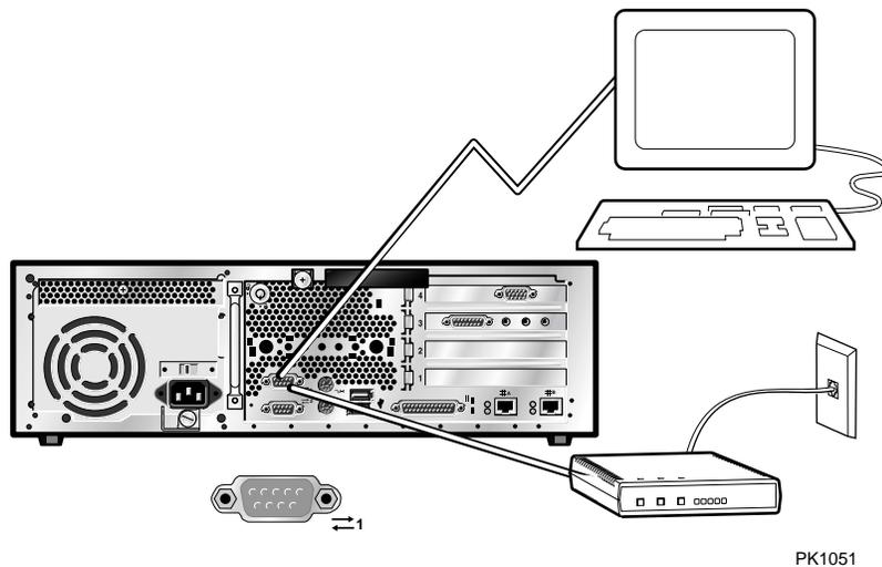
You can connect a terminal or a modem to the COM1 port, but not both at the same time. You use the terminal to set RMC parameters for the connection, then connect the modem. See Section 4.9.
