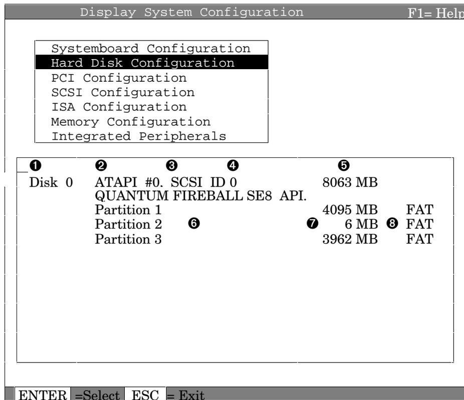
*NOTE: This screen is for information only; it cannot be edited. To make changes to the hard disk setup, use the **Hard Disk Setup** screen.*
