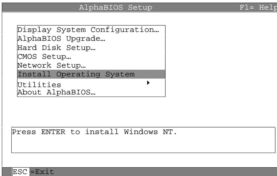
If Windows NT was installed at the factory, Windows NT setup will start automatically the first time the system powers up.
