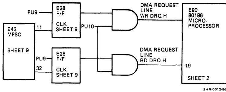
Figure 6-6 DMA Channel (MP-2059, CS, Sheets 2 and 9)
