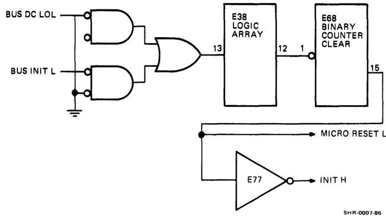
Figure 6-1 Power Up Reset Circuitry
