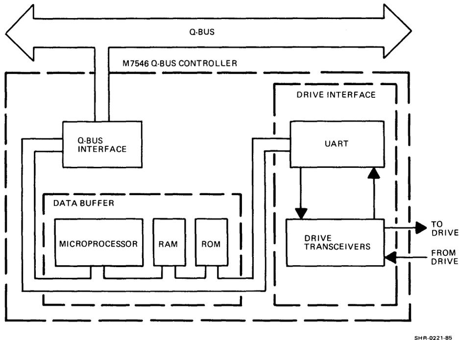
Figure 5-1 TQK50 High Level Block Diagram
