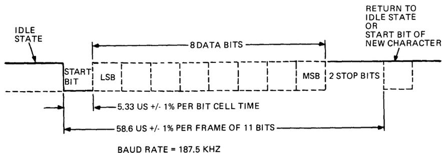
Figure 2-11 Frame Format of Data Coming from Controller
