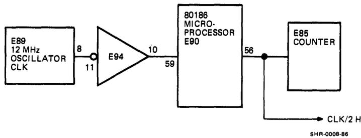
Figure 6-2 Microprocessor Timing Circuit
