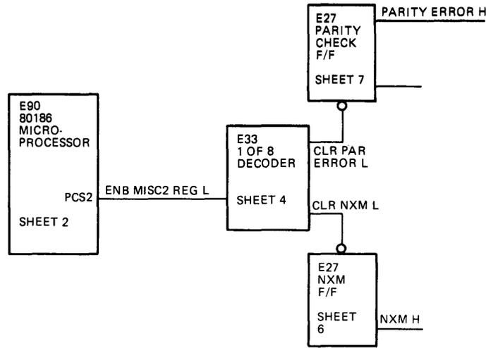
Figure 6-5 FPLS Interrupt (MP-2059, CS, Sheets 2, 4, 6, & 7)
