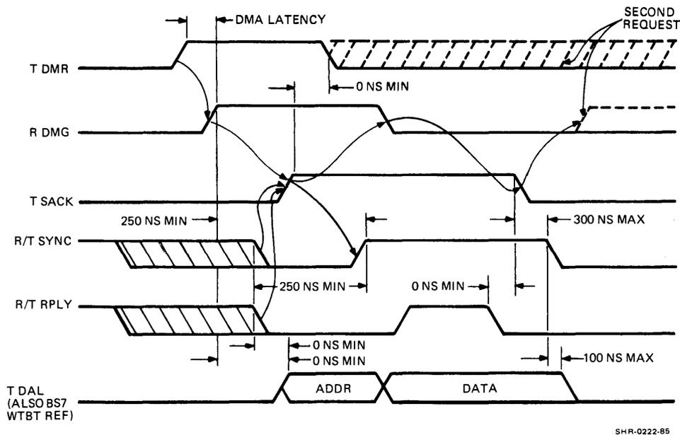
Figure 5-2 Q-bus Timing
