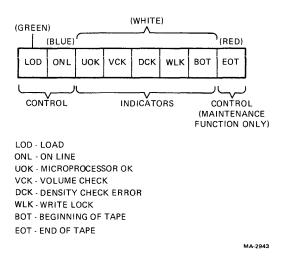
Figure 4-1 TS11 Transport Controls and Indicators
