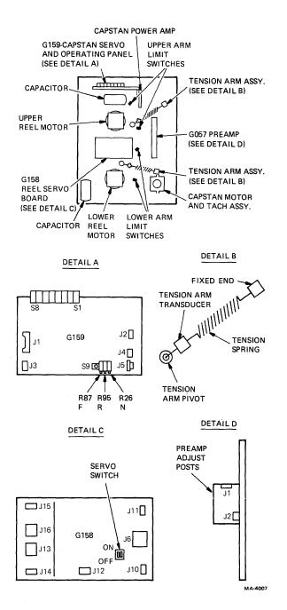
Figure 1-4 Transport Assemblies (Rear View)
