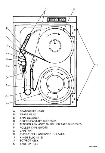
Figure 4-3 Tape Loading Path
