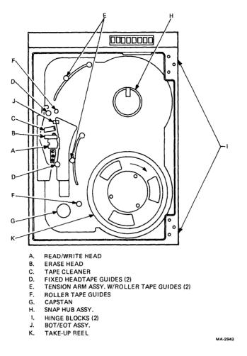
Figure 3-1 Transport Components to Be Cleaned
