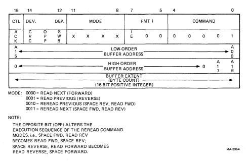
Figure 5-9 Read Command Packet Example
