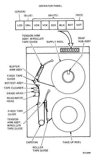
Figure 1-3 Transport Assemblies (Front View)
