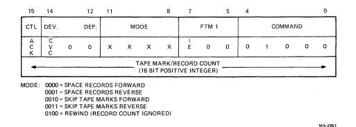
Figure 5-12 Position Command Packet Example
