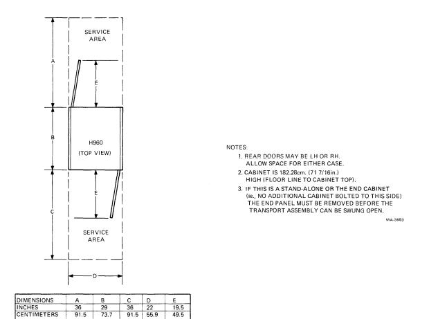
Figure 2-1 Space and Service Clearance, H960 Cabinet and Rackmount (Top View)
