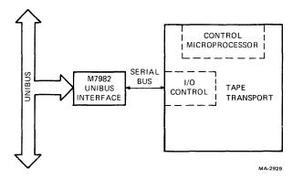
Figure 1-1 TS11 Subsystem Configuration
