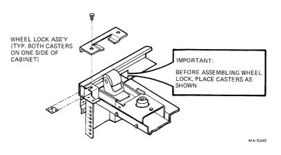
Figure 2-8 Caster Lock Assembly
