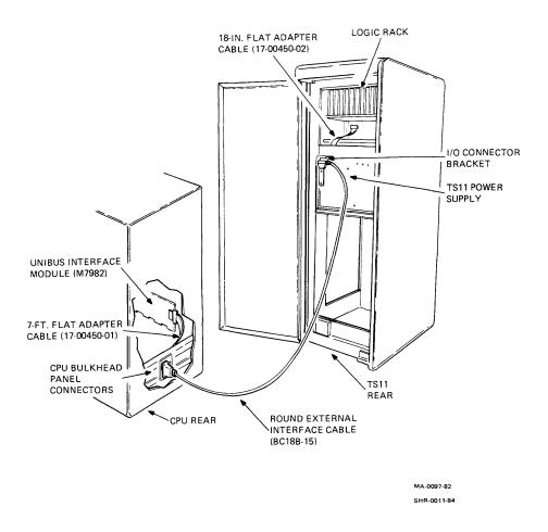
Figure 2-13 TS11 Signal Cabling
