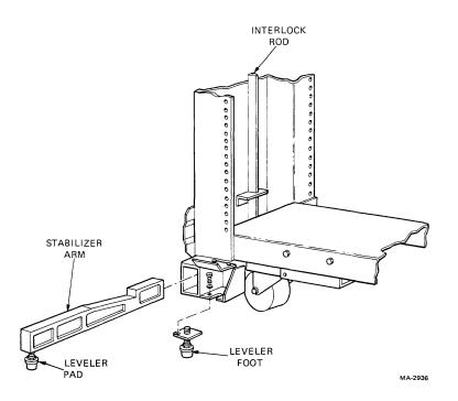
Figure 2-7 H9602 Stabilizer Leg and Leveler Feet Locations
