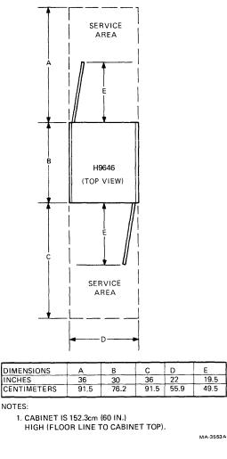
Figure 2-3 Space and Service Clearance, H9646 Cabinet (Top View)
