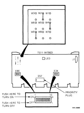
Figure 2-12 M7982 Interface Module
