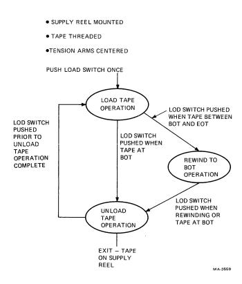
Figure 4-2 Load Switch State Diagram
