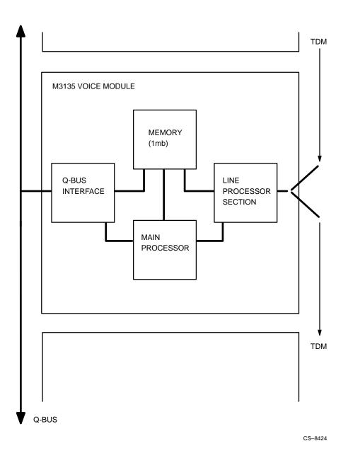
Figure 18 Functional Block Diagram of the M3135 Voice Module
