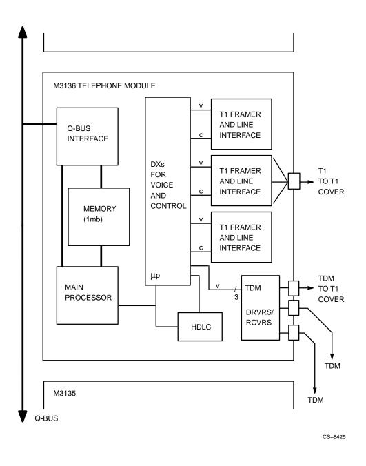
Figure 2 Functional Block Diagram of the M3136 Module
