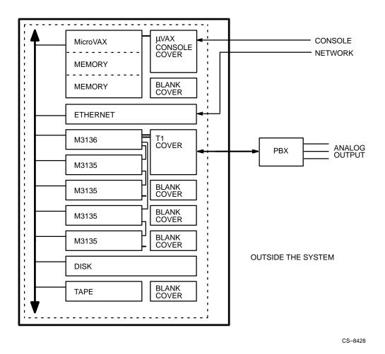
Figure 1 Functional Block Diagram of the DECvoice-T1 System (continued)
