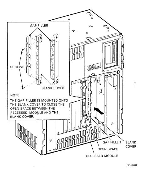
Figure 13 Gap Filler Installation
