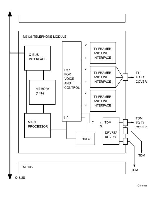
Figure 17 Functional Block Diagram of the M3136 Telephone Module
