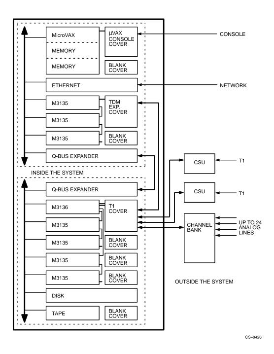
Figure 1 Functional Block Diagram of the DECvoice-T1 System
