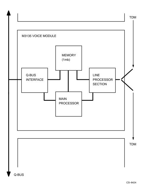
Figure 3 Functional Block Diagram of the M3135 Module
