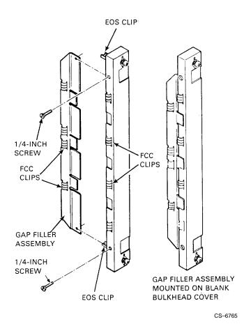
Figure 14 Attaching the Gap Filler Assembly
