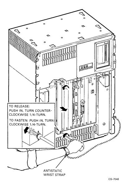
Figure 9 Releasing the Captive Screws
