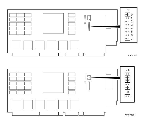
Figure 9-8 shows jumper locations for the CDROM drive.
