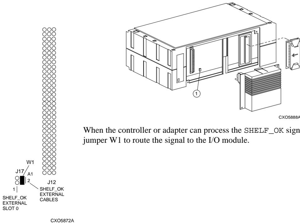
When the controller or adapter can process the SHELF\_OK signal, install jumper W1 to route the signal to the I/O module.
