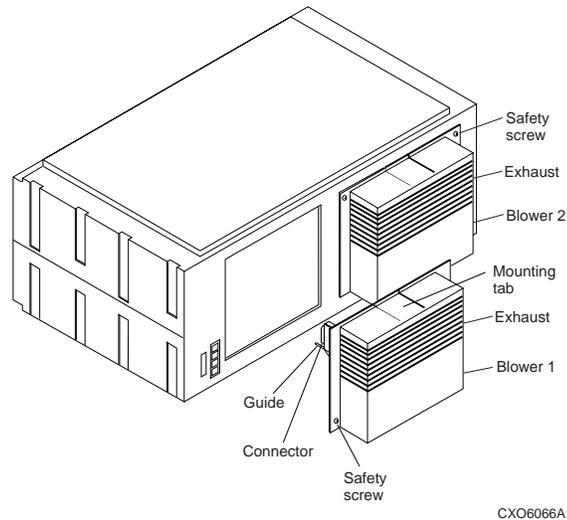
6. Align the replacement blower connector and push the blower straight in, making sure that both mounting tabs lock in place.
