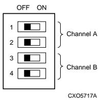
1. The top two switches (S4–1 and S4–2) control termination for channel A on both single-channel and dual-channel, I/O modules.
