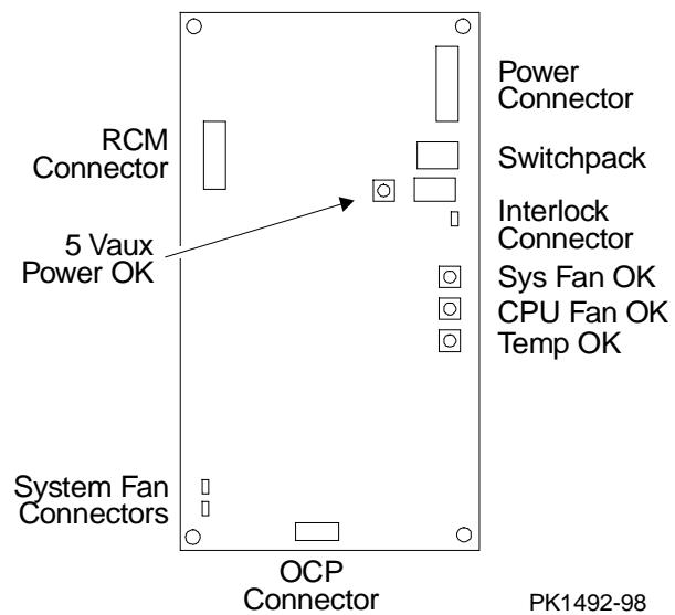
The system allows both local and remote control. The remote control firmware and a set of switches that enable or disable remote control features reside on the server feature module.
