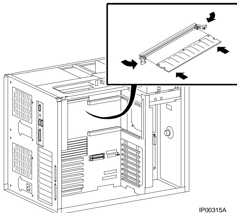
*WARNING: CPU modules and memory DIMMs have parts that operate at high temperatures. Wait 2 minutes after power is removed before touching any module.*
