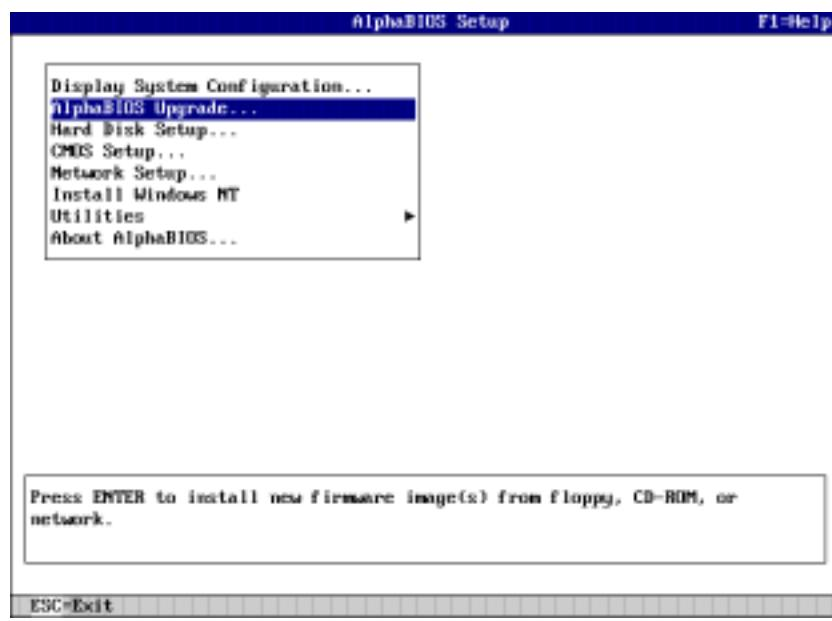
Use the Loadable Firmware Update (LFU) utility to update system firmware. You can start LFU from either the SRM console or the AlphaBIOS console.
