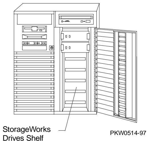
The StorageWorks drives are to the right of the system cage. Up to seven drives fit into the shelf. The system supports fast wide UltraSCSI disk drives. The RAID controller is also supported. With an optional UltraSCSI Bus Splitter Kit, the StorageWorks shelf can be split into two buses.
