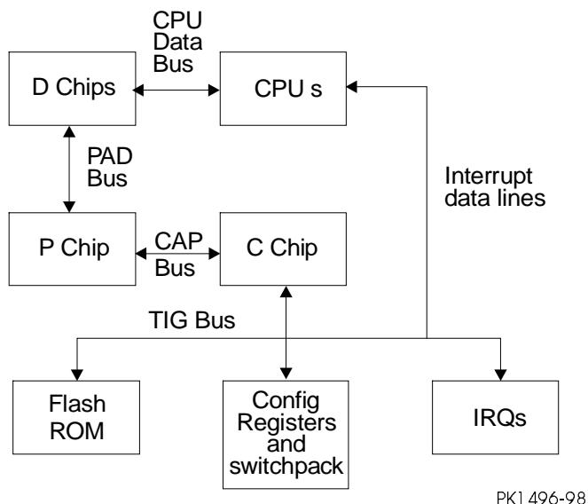
Figure 1-18 is a block diagram of the TIG bus implemented through the TIG chip. Three system functions are carried out on this bus.
