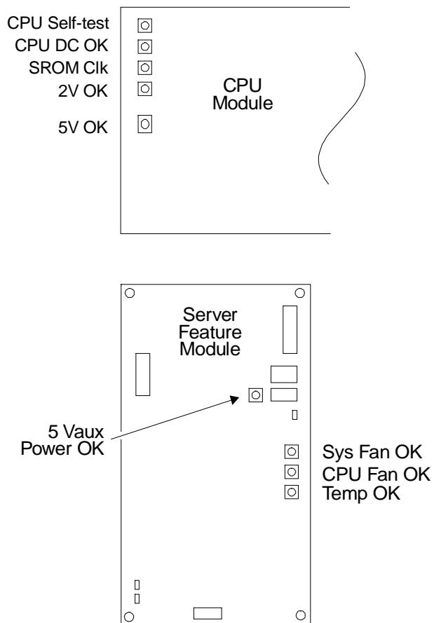
To see LEDs, the card cage side of the system must be exposed; the system top should be on, and the system must be on.
